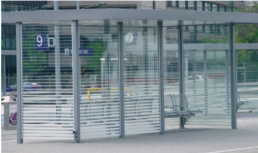
Bus shelters, small noise protection barriers, wind barriers and balcony balustrades, etc. can also be easily retrofitted with vertical or horizontal stripes. This shelter in Munich was constructed with printed stripes.
