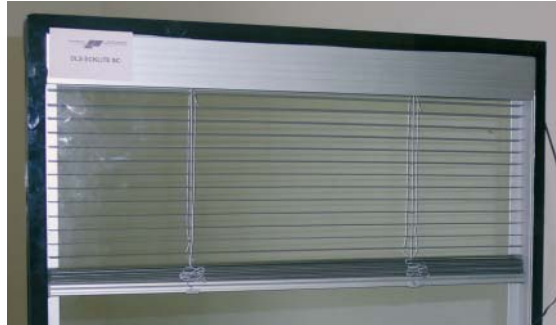
Embedded blinds. When in use, even if set at an angle, they provide a degree of protection.
