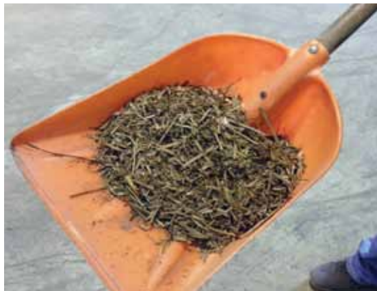
Photos above: Chełm cement plant, shredding biomass to be used as fuel; Shredded biomass - J. Krogulec
