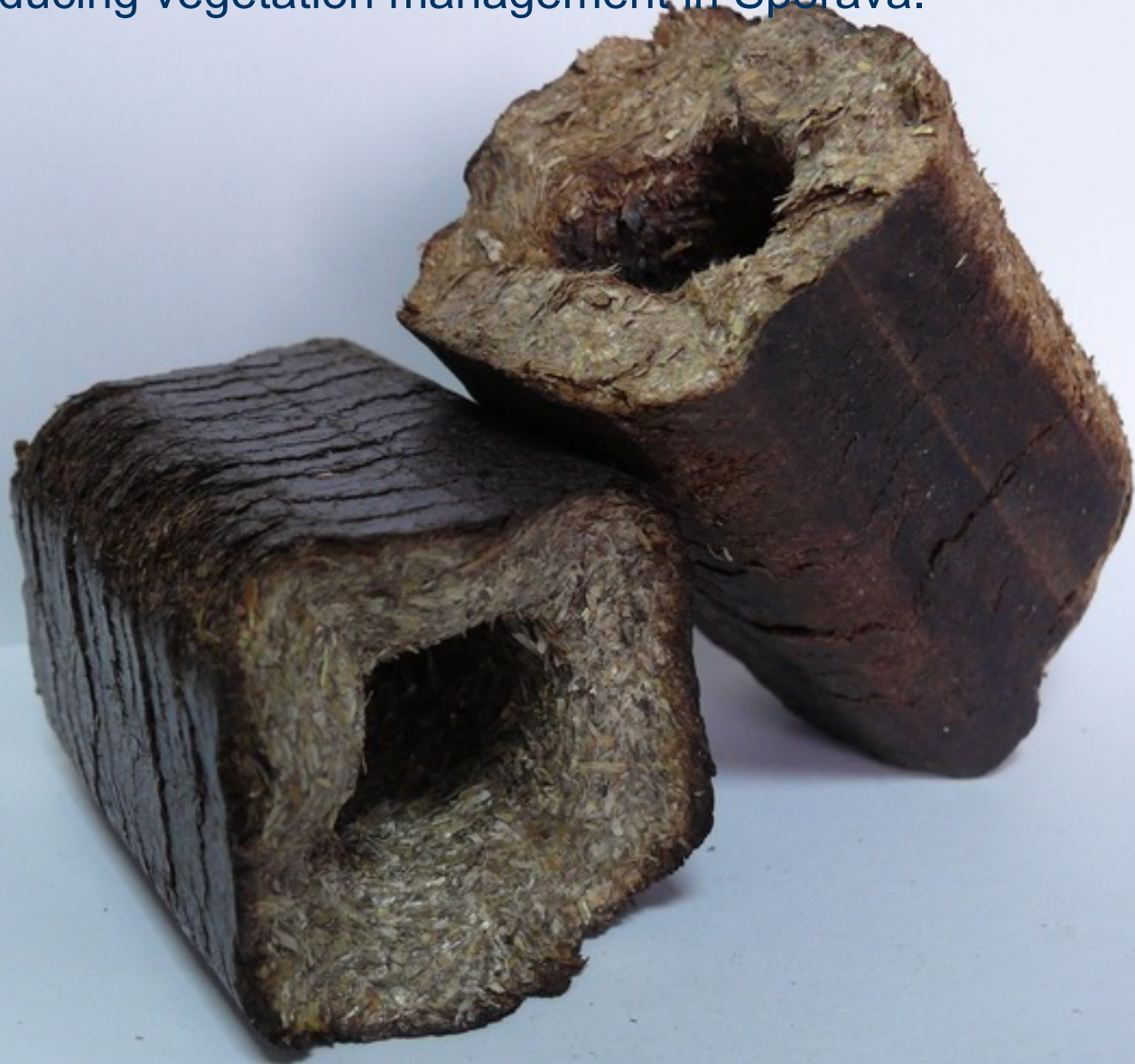
Trial briquettes produced out of biomass harvested in Sporava (2010)
