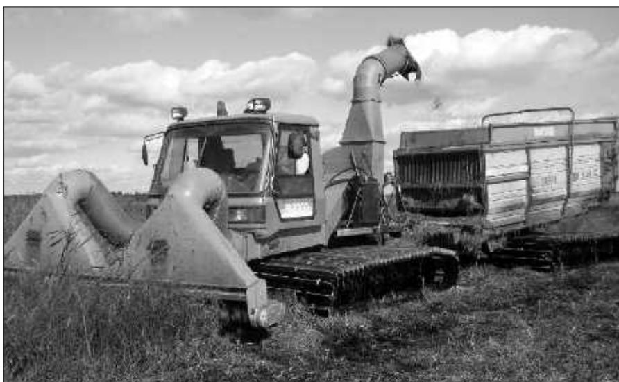
Fig. 12: Prototype mowing equipment used to manage peat meadows in the Biebrza Valley since 2007. (Photo: Lars Lachmann)
