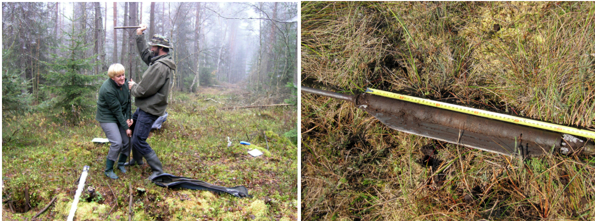
Peat drilling is the standard, not omittable method of recognising both peatland history and the present condition of the peat.
