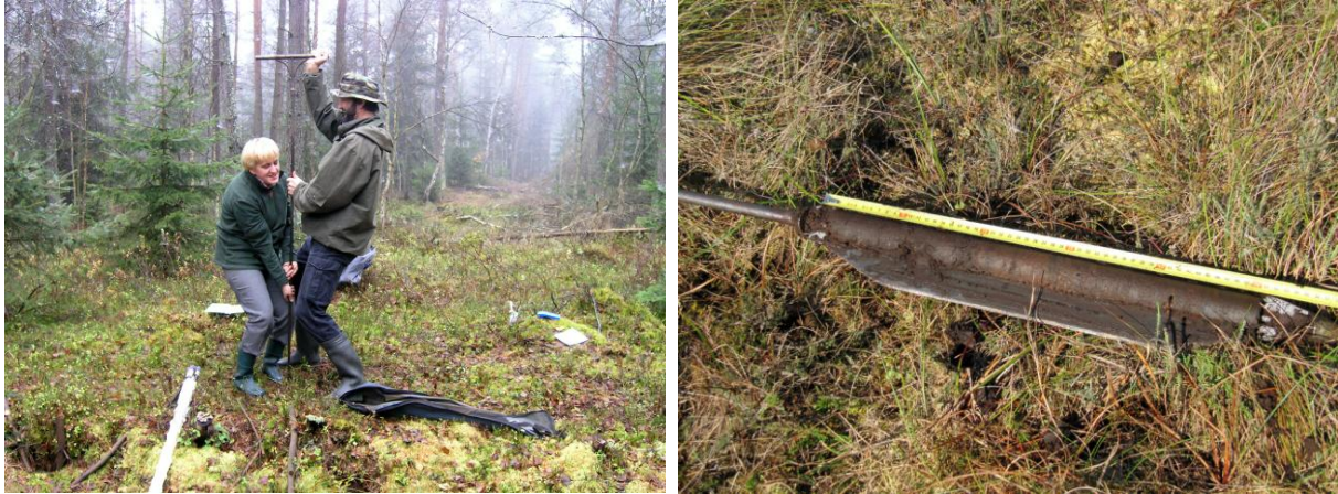
Peat drilling is the standard, not omissible method of recognising both peatland history and the present condition of the peat.
