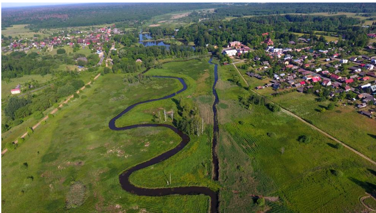
Restored Narewka river in Białowieża (credit Edyta Kapowicz). Re-creating river meanders was followed by significant valley fen rewetting.
