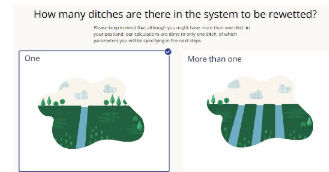
Figure 1.3. SERVIPEAT dialog window in the simplified mode – selection of calculation path that depend on the number of drainage ditches in the system to be rewetted.
